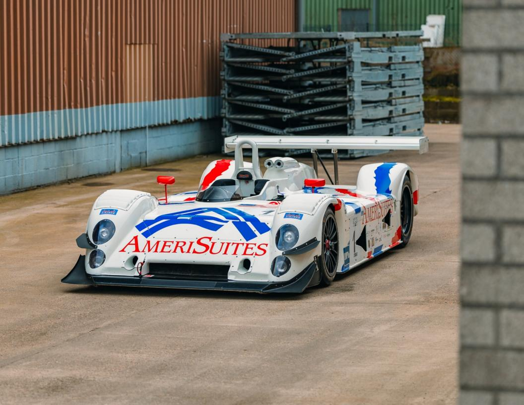
As the rate of development in the top-flight LMP900 category of sports car racing rose, Riley & Scott produced a new car dubbed the Mk3C. Building on the proven Mk3 package, the new Mk3C incorporated some of the lessons learnt in the Riley & Scott developed Cadillac Northstar LMP.
